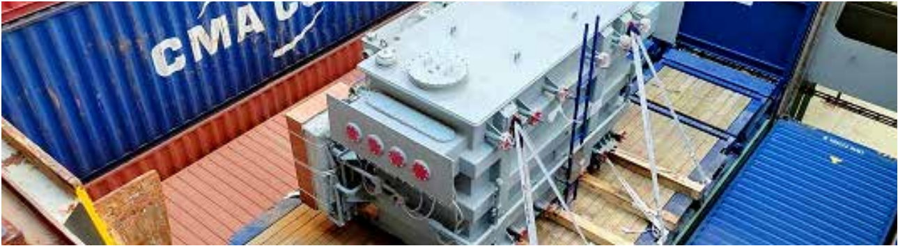
230kV Three Phase Power Transformer in Nevada
